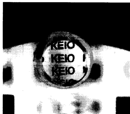
Fig. 7. Photograph of the reversed real image formed on the surface of the quarter pitch length MMA-BEN system GI preform. Diameter: 16 mm.
